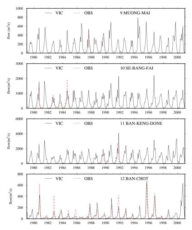
Figure 4.13 Comparison of VIC simulated monthly streamflow [solid line] and observed streamflow [broken line] at stations 9, 10,11 and 12 of Figure 4.6
