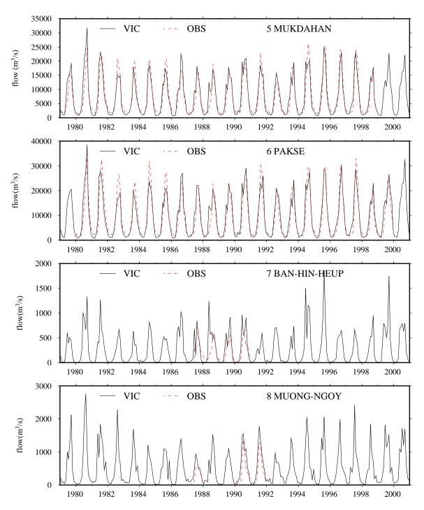
Figure 4.12 Comparison of VIC simulated monthly streamflow [solid line] and observed streamflow [broken line] at stations 5, 6, 7 and 8 of Figure 4.6
