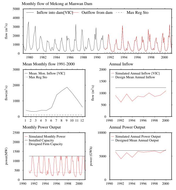
Figure 4.16 MWMM output for Manwan Dam [Dam 1 in Figure 4.15]
