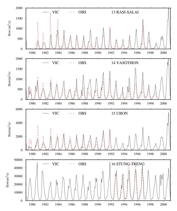
Figure 4.14 Comparison of VIC simulated monthly streamflow [solid line] and observed streamflow [broken line] at stations 13, 14, 15 and 16 of Figure 4.6
