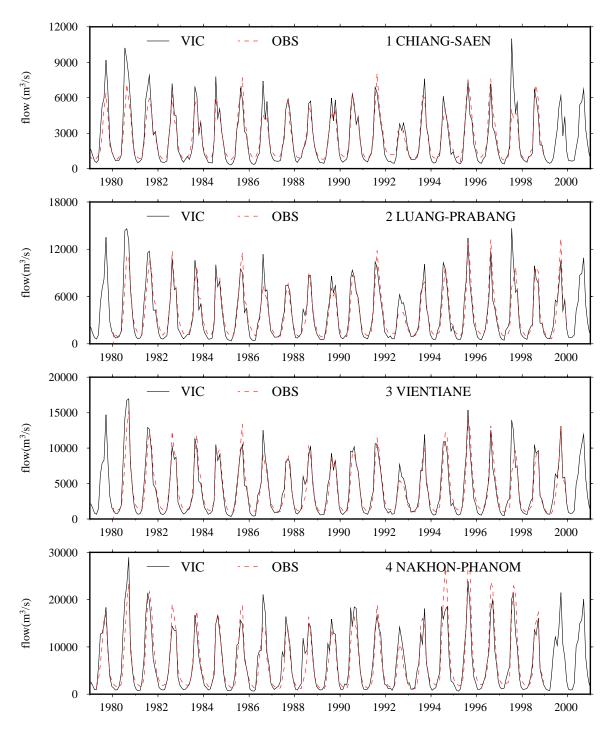
Figure 4.11 Comparison of VIC simulated monthly streamflow [solid line] and observed streamflow [broken line] at stations 1, 2, 3 and 4 of Figure 4.6
