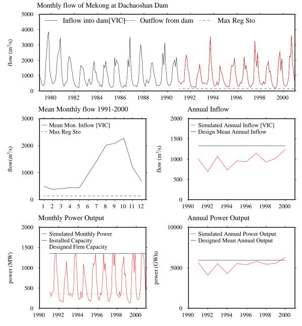
Figure 4.17 MWMM output for Dachaoshan Dam [Dam 2 in Figure 4.15]
