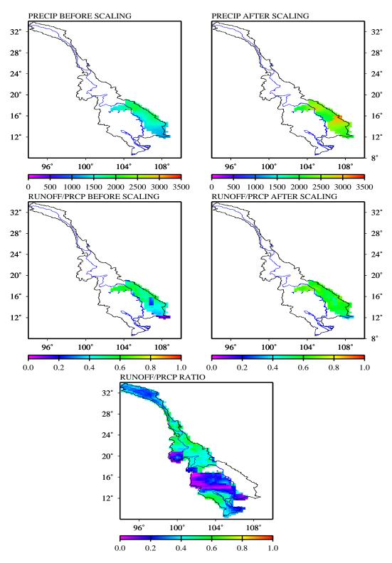
Figure 4.10 Effect of scaling precipitation data on precipitation and runoff
