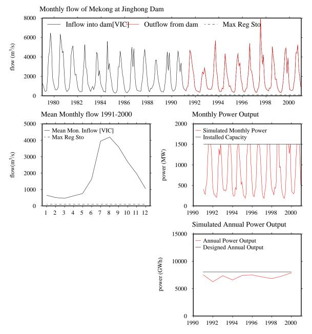
Figure 4.21 MWMM output for proposed Jinghong Dam [Dam 6 in Figure 4.15]
