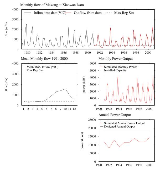
Figure 4.22 MWMM output for proposed Xiaowan Dam [Dam 7 in Figure 4.15]
