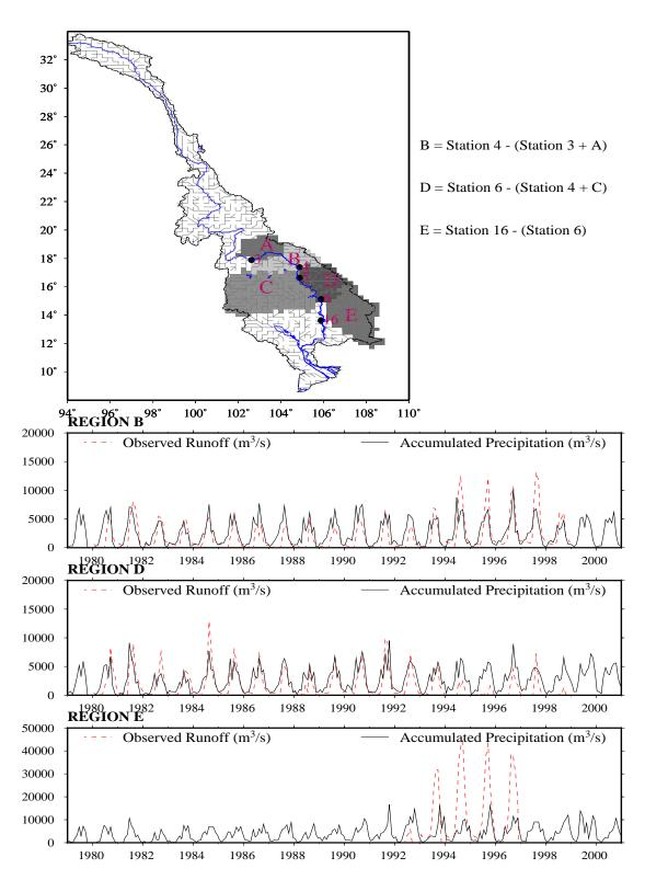
Figure 4.9 Comparison of observed runoff and accumulated precipitation for regions B, D and E
