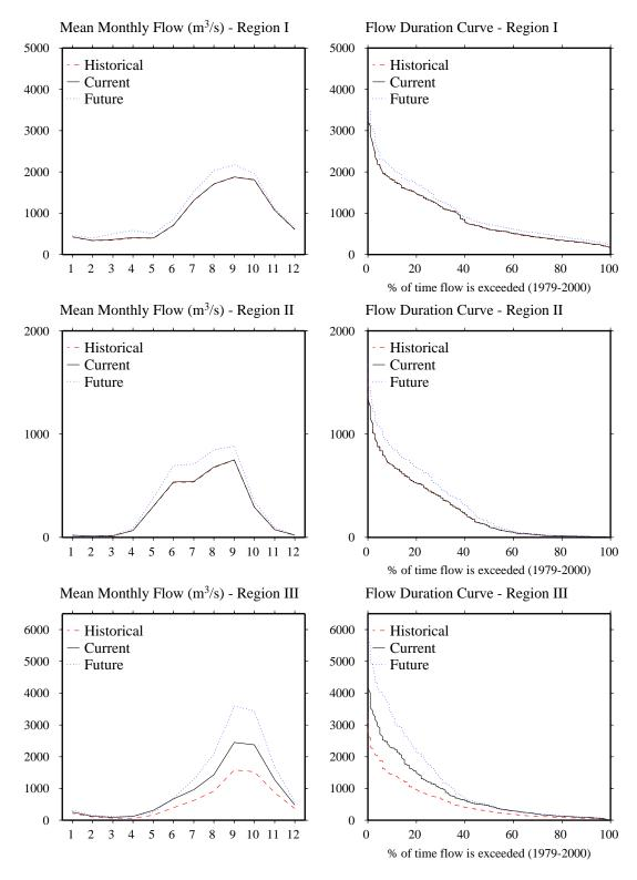
Figure 5.3 Mean monthly streamflow generated using HLC and FLC for all the three regions
