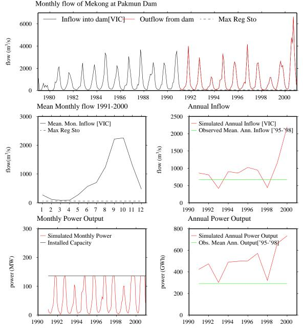
Figure 4.20 MWMM output for Pak Mun Dam [Dam 5 in Figure 4.15]
