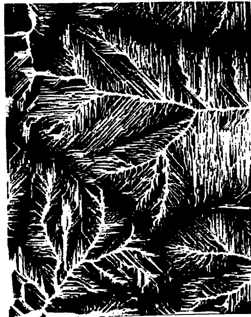
Figure 16. Image of the SCA matrix for the Mettman Ridge study area obtained with D8. A logarithmic scale of gray shades is used; lighter shades correspond to higher values.
