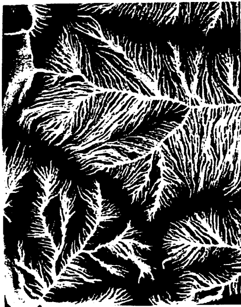
Figure 14. Image of the SCA matrix for the Mettman Ridge study area obtained with DEMON. A logarithmic scale of gray shades is used; lighter shades correspond to higher values.
